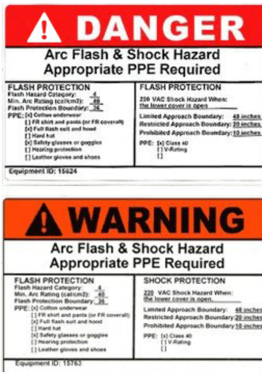
Figure 5-6 – Arc Flash Warning Labels (Typical)
